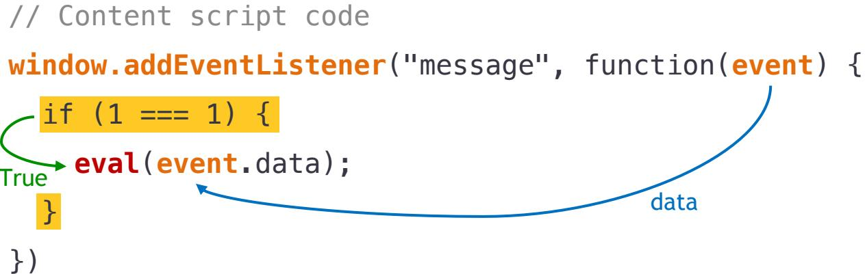
The diagram illustrates data flow analysis on the provided JavaScript code. A blue curved arrow labeled 'data' points from the variable 'event.data' in the code to the 'eval' statement. A green curved arrow labeled 'True' points from the condition '1 === 1' to the start of the if-block. The code itself is displayed in a light gray background, while the annotated parts are highlighted in yellow boxes.
